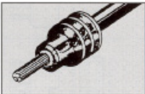
2. Align seal with cable insulation.
