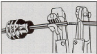
1. Apply seal to cable before stripping insulation.
